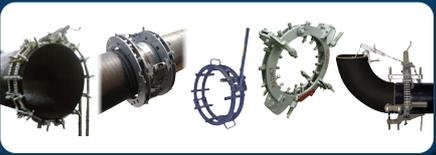
With continuous improvement and new additions, Mathey Dearman is now offering the most complete line in the industry of pipe alignment and reforming clamps.
