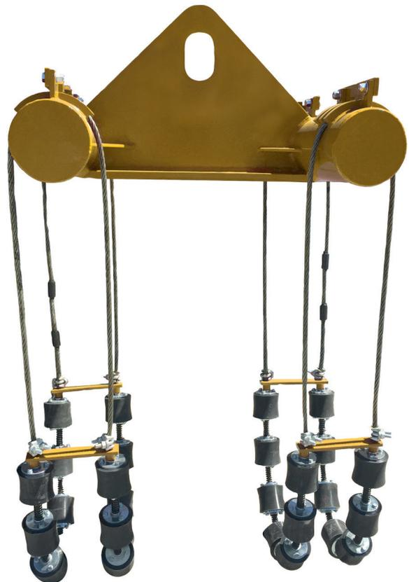
Mathey Dearman's Pipe Cradles and Slings are an effective way to move pipe, specifically designed for pipeline installation projects. Mathey Dearman currently offers cradles from 2" - 36" and all are equipped with 4 inch urethane "round cut" wheels with sealed anti-friction bearings. All spreader bar designs are third party tested and comply with industry standards. These models are equipped with 5/8" wire rope and all rope is swaged and certified.
