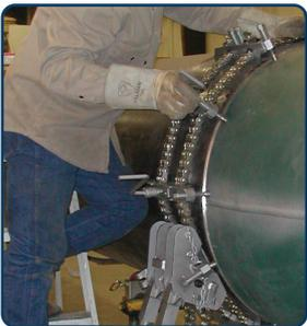
Joints on large pipe or tube shells up to 240" (6,096 mm) in diameter can be aligned, reformed and welded without removing the clamp, saving time and improving weld quality.
