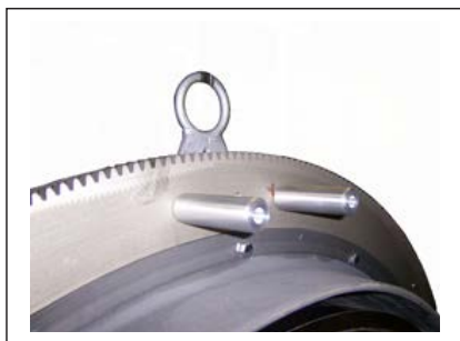
Picture 5 – Installation of Extension Plate Spacer
