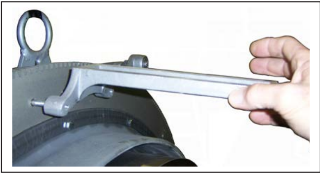
Picture 3 – Installation of Torch Arm on the Threaded Stud
