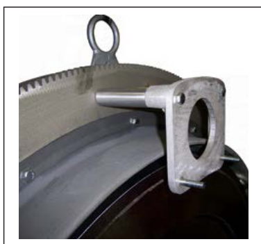
Picture 6 – Extension Plate Attached to Extension Plate Spacer
