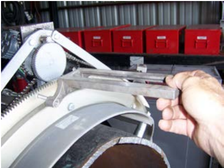
Picture 3 – Installation of Torch Arm on the Threaded Stud
