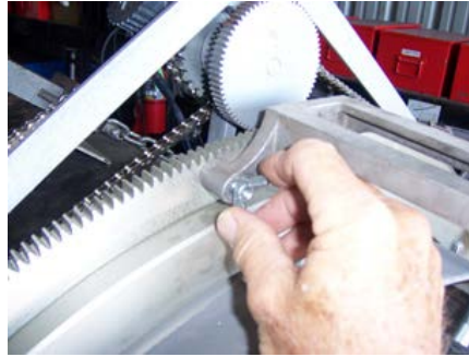
Picture 4 – Installation of the Wing Nut
