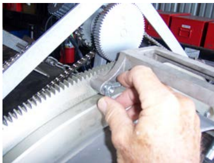
Picture 5 – Installation of the Wing Nut
