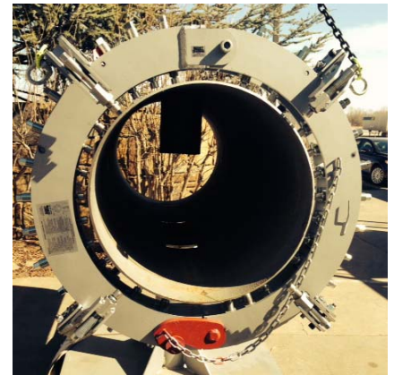
Figure 5 - Rim Clamp secured on pipe.
