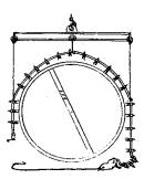
Approximately dimensions of the spreader bar cable for use on 15' diameter vessel: center cable 2' long, end cables 9'6" long. When hooking to the clamp, space hook at 11'7" from center of hook.
