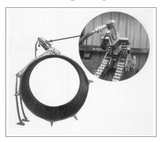
Large Diameter Double Chain Clamps may have one or more Main Block Assemblies depending on the clamping range of the Clamp in order to properly and uniformly take up the slack in the Chain. Each section of the clamp will have a Main Block and Fine Adjustment to remove the slack in the chain. Multiple Main Blocks enable the operator to remove the slack in a section of the chain. The use of Multiple greatly aids in the installation, application and function of the clamp.
