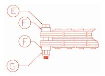
2. Run the end of the Roller Chain from which items E, F and G were removed through the bottom side of the Main Block and underneath the chain dog.
