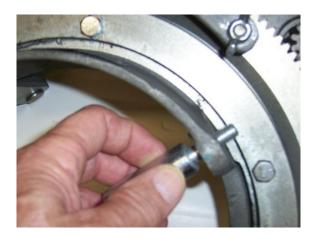
Picture 2 - Installation of Spacer Bolt
