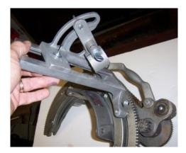
Picture 5 - Installation of Torch Arm on Threaded Stud
